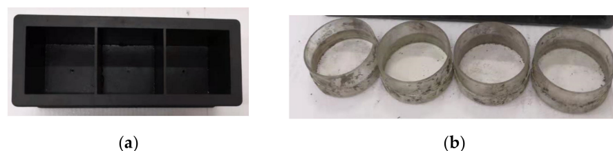
Figure 2. Specimen preparation molds (a) cube molds; (b) cylinder molds.
