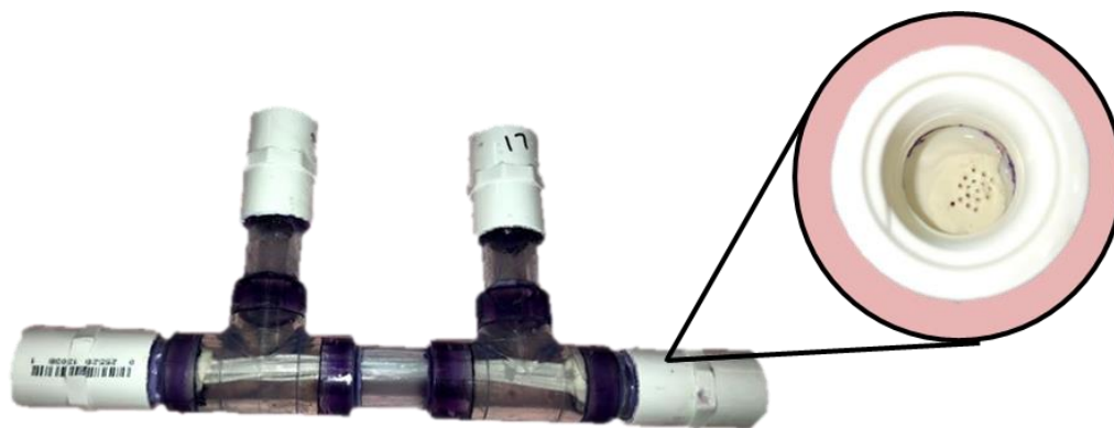
Figure 2. Example of the hemodialysis module used for running tests.
