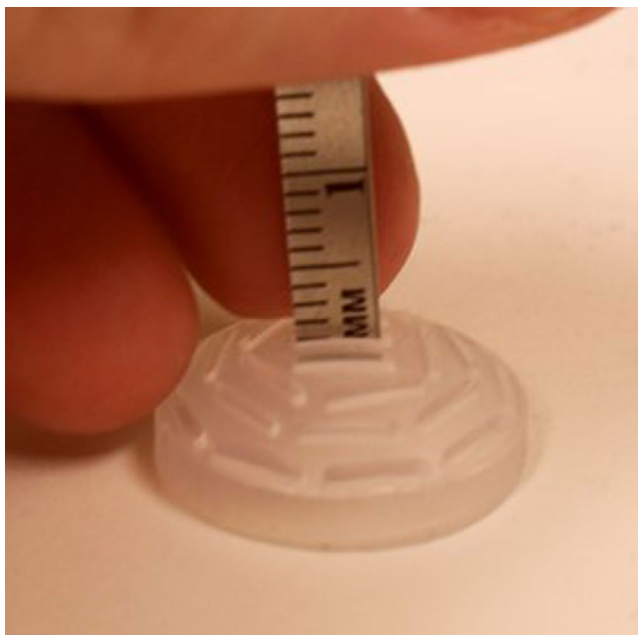
FIGURE 9 An inexpensive slot depth measurement tool was made by cutting a metal ruler lengthwise to fit in the narrow seed slot depth. The tool was used to ensure slot depths were 1.25 \pm 0.5 mm by verifying that the slot is nearly 1.25 mm
