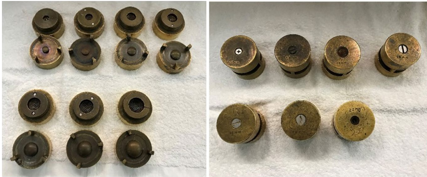
FIGURE 2 The seven brass molds that have been used to produce all COMS Silastic inserts to date are shown. Left: Open molds, Right: Closed molds
