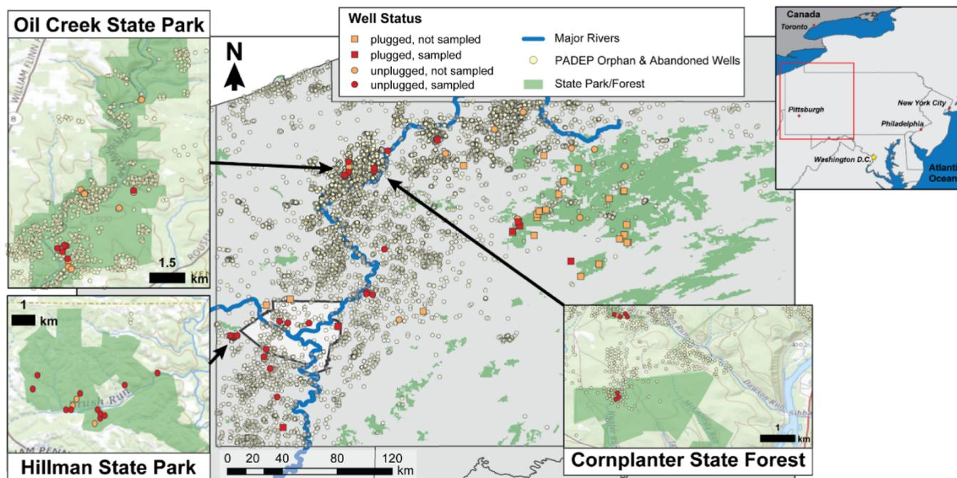
**Figure 1.** Locations of documented abandoned wells in western Pennsylvania having coordinates,<sup>2</sup> plugged and unplugged abandoned wells screened but not sampled in this investigation, and plugged and unplugged abandoned wells both screened and sampled in this investigation. State park<sup>5</sup> and state forest<sup>6</sup> boundaries are included where screening and sampling occurred. The polygon in southwestern Pennsylvania represents the outline of Allegheny County.
