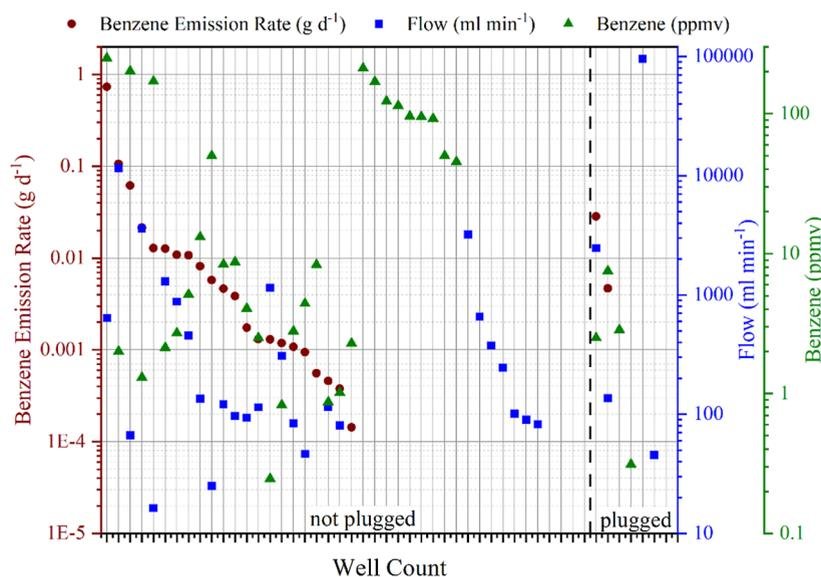
**Figure 3.** Emission rates for benzene when detectable flow and benzene concentrations are present, detectable concentrations of benzene, and detectable flow rates (plotted in this order) for unplugged and plugged abandoned wells in western Pennsylvania. Wells with both non-detectable flow and benzene concentrations are left blank.
