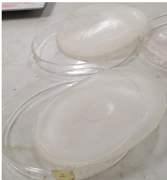
Figure 2. Nano-calcium carbonate reinforced polylactic acid films.
