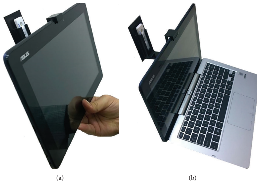
FIGURE 3: (a) A view of a tablet and worn RDT holder. (b) A view of a laptop and worn RDT holder.
