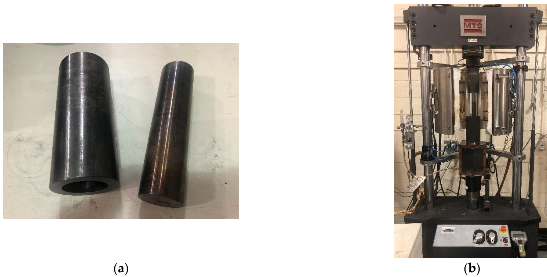
Figure 1. Device for the compaction of the anode paste. (a) Rigid die; (b) MTS Servohydraulic press.
