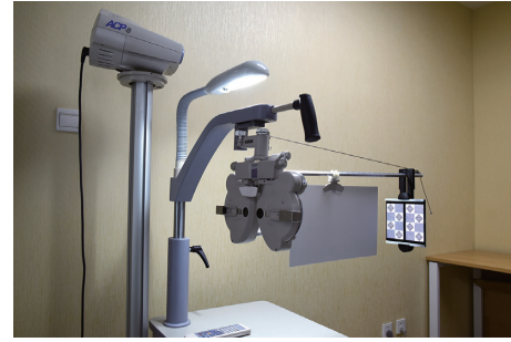
FIGURE 1: The test system used consisted of a phoropter and two Sony smartphones. A pair of smartphone pictures are seen with a black and white pattern.
