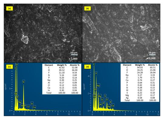
**Figure 7.** The images of SEM and EDS spectra of (**a**, **c**) unmodified membrane and (**b**, **d**) AgNPs-MF membrane after 60 days in submerged mode.
