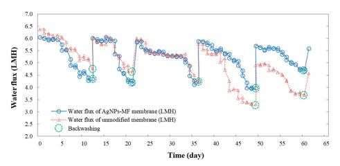
**Figure 4.** The comparative study of permeate flux of the unmodified membrane module and the AgNPs-MF membrane module over the 60-day operation period.
