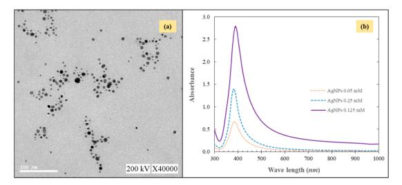
Figure 1. TEM image (a) and (b) UV-vis absorption spectrum of the AgNPs.
