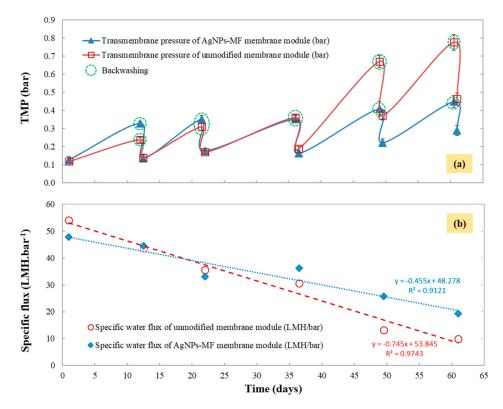
**Figure 5.** The variation of (**a**) transmembrane pressure (TMP) and (**b**) specific flux variation for the unmodified membrane module and the AgNPs-MF membrane module.
