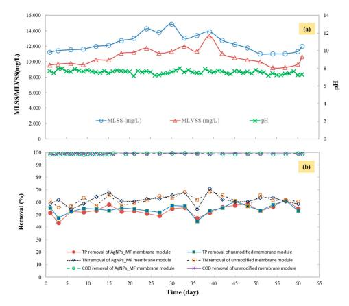
**Figure 3.** MF-MBR performance in terms of: (a) Operation condition, (b) removal of Chemical Oxygen Demand (COD), total nitrogen (TN) and TP of unmodified membrane module and the AgNPs-MF membrane module. The dissolved oxygen and temperature of the bioreactor were maintained in the range of  $3-4 \text{ MgO}_2/\text{L}$  and  $25-30 \,^{\circ}\text{C}$ , respectively.
