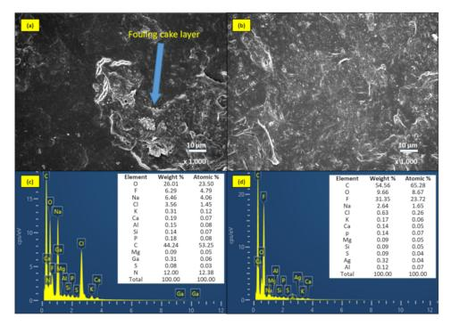
**Figure 6.** The images of SEM and EDS spectra of (**a**, **c**) unmodified membrane and (**b**, **d**) AgNPs-MF membrane after 60 days in operation mode.
