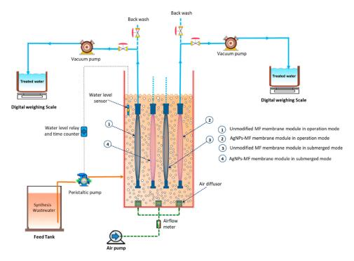
Figure 9. Schematic of the experimental setup for lab-scale MF-MBR system.
