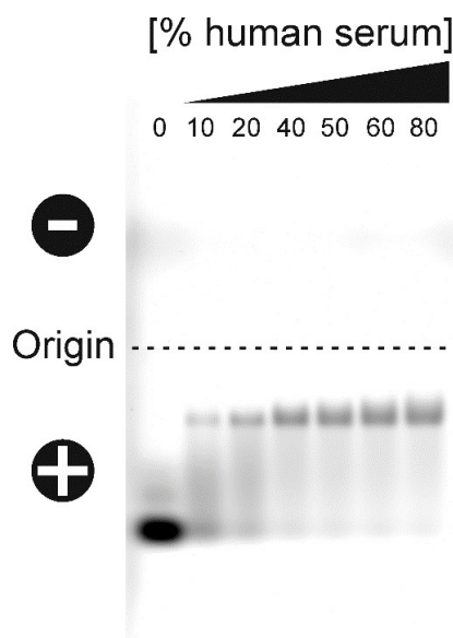
Figure 7. Effect of human serum on the electrophoretic mobility of FITC-labeled, alendronate-containing \text{BaSO}_4 NPs. Increasing concentrations of human serum were incubated with NP concentrations of 0.1 \mu\text{g}/\mu\text{L} for 1 h at 37^\circ\text{C} . Afterwards, the biomolecule-NP-complexes were separated by electrophoresis on a 1% TAE-agarose gel (pH 8). Fluorescence signals originating from FITC-labeled NPs were finally documented using a Typhoon fluorescence scanner. The percentage denotes the concentration of human serum used for incubation.
