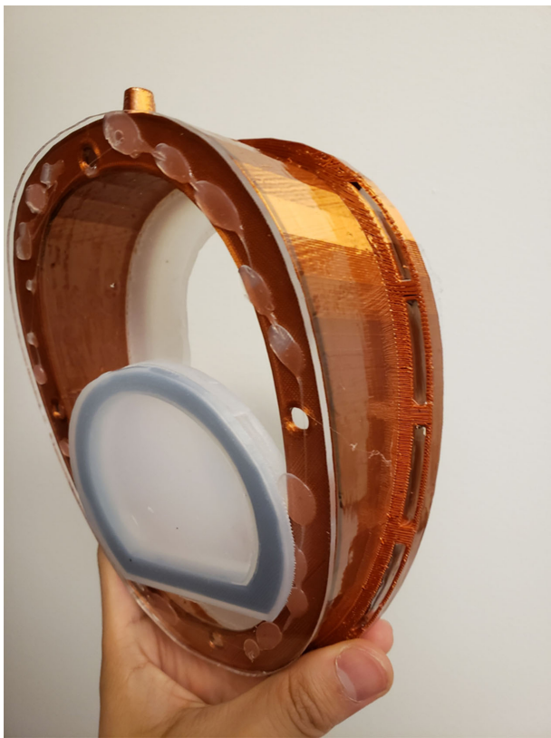
FIGURE 1. Front view of device showing 3D-printed poly(lactic acid) (PLA) frame, transparent acrylic shield, and semicircular instrument port with silicone diaphragm.
