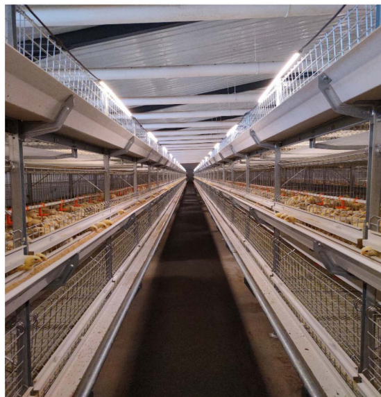
Figure 1. Structure of broiler house and waterline system.
