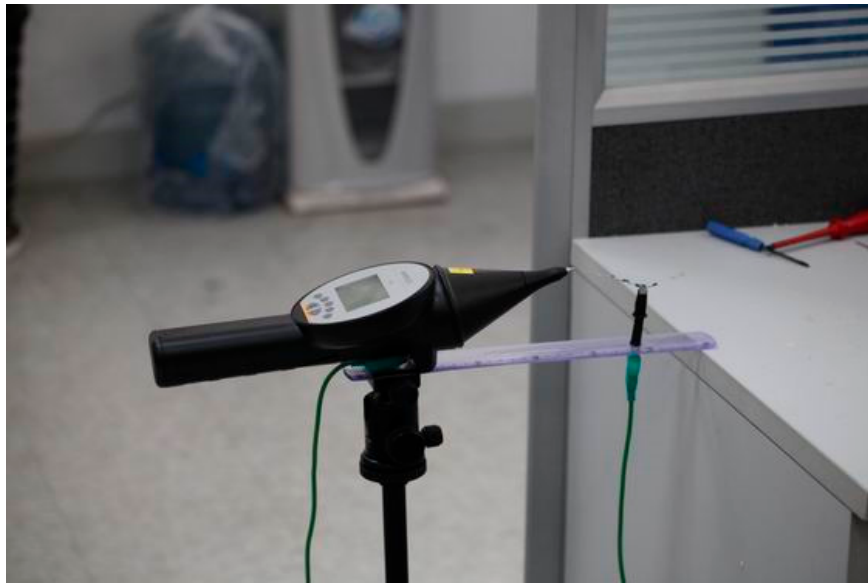
Figure 11. The PD simulator “EM TEST DITO”.
