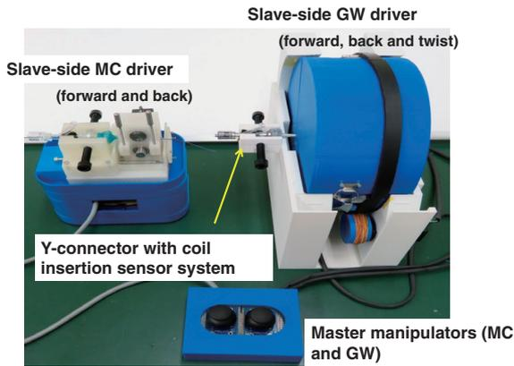
**Fig. 3** Neuroendovascular intervention support robot system. GW, guidewire; MC, microcatheter
