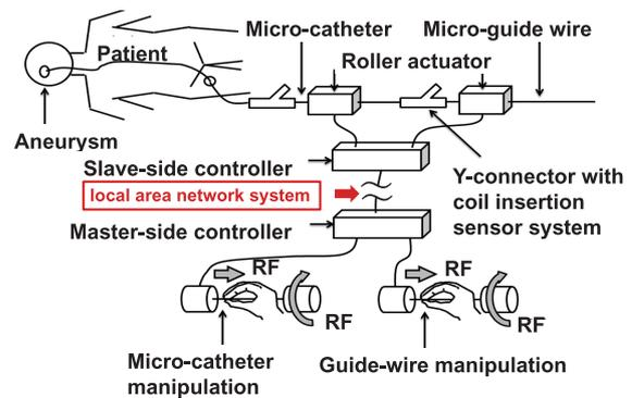
**Fig. 4** Scheme of control mechanism of neuroendovascular intervention support robot system. RF, reaction force
