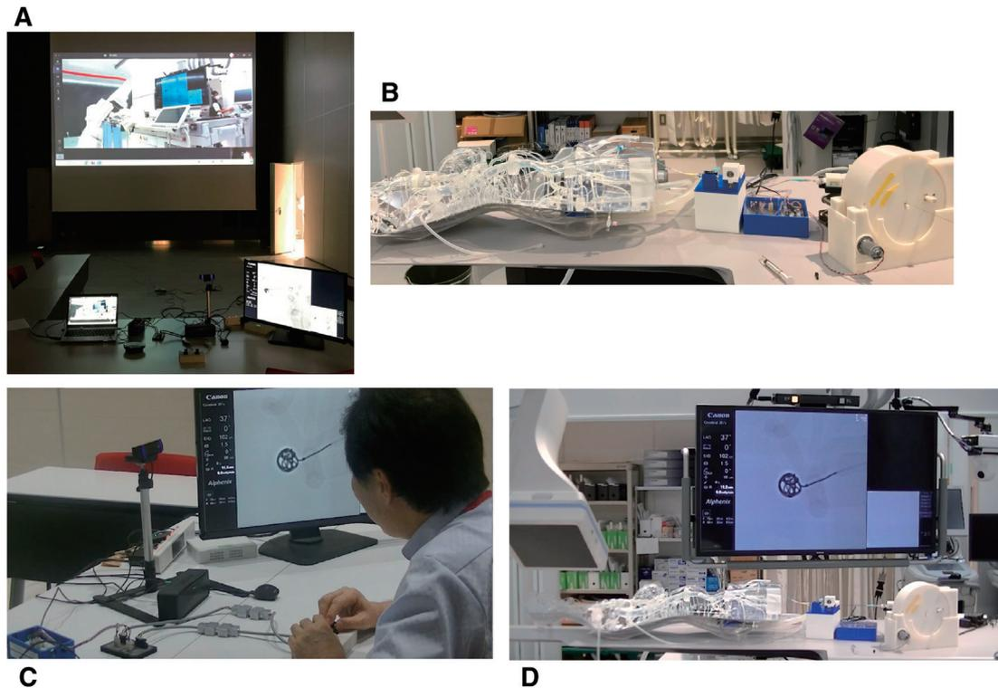
**Fig. 5** Remote experimental telesurgery of aneurysm embolization. Master control room (A) is located 50 m from the angiography room (B), where the vascular model and slave robot are set on the table. The coiling operation on the master side (C) corresponded exactly with the operation on the slave side (D).
