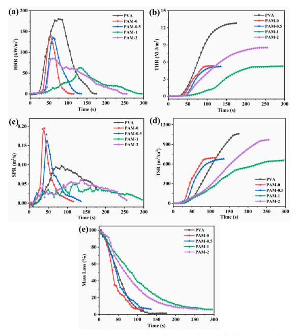
**Figure 5.** HRR (**a**), THR (**b**), SPR (**c**), TSP (**d**), and mass loss (**e**) as a function of the burning time for PVA and its composite aerogels.
