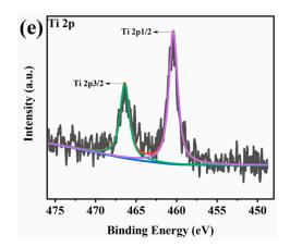
Figure 12. (a) C 1s, (b) O 1s, (c) N 1s, (d) P 2p, and (e) Ti 2p XPS spectra of the residues for PAM-1.
