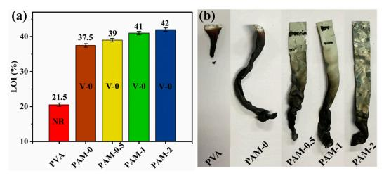
**Figure 4.** (a) LOI, UL-94 test results and (b) the photos of the char residues after UL-94 test for pure PVA and its composite aerogels.
