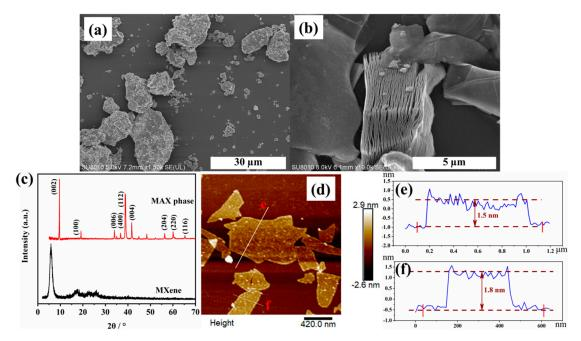
**Figure 1.** (a) SEM image of MAX phase; (b) SEM image of non-stripped MXene in low resolution; (c) XRD image of MAX phase and MXene; (d–f) AFM image of stripped MXene and the corresponding height profiles.
