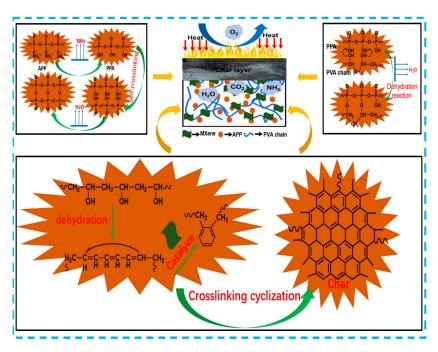
**Scheme 2.** Schematic illustration for the synergistic flame-retardant mechanism of PVA-APP-MXene composite aerogels.
