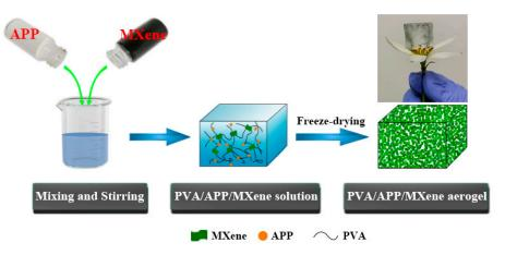
Scheme 1. Preparation process for PVA/APP/MXene composite aerogel.
