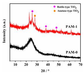
Figure 9. XRD patterns of the char residues of PAM-0 and PAM-1 composite aerogels.
