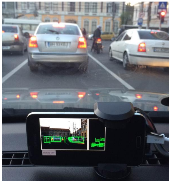
Figure 17. Obstacle detection on the Samsung Galaxy S5 smartphone: Stop and go traffic.
