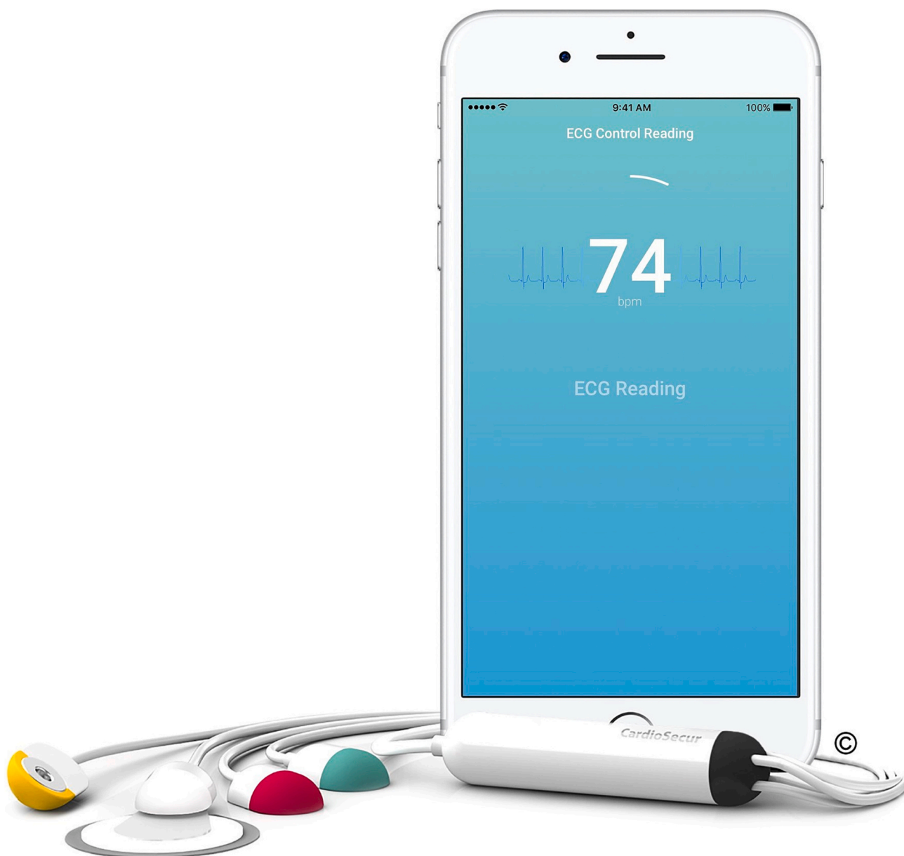
Fig. 1. Picture of the mobile "CardioSecur" ECG system.
