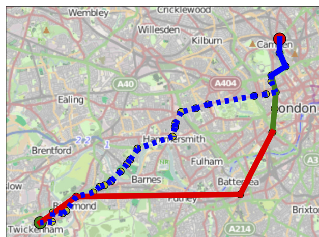
Figure 1 | Example of the difference between a time-respecting path (solid line) and a minimal path (dashed line). Here, we show a trip from Twickenham to Camden Town in London, and the minimal path would use only buses (marked in Blue). The optimal time-respecting path in this case is remarkably multi-modal: the bus layer is still used for the final segment, which is the same as for the minimal path, while the Rail layer (Red) and then the Metro layer (Green) are used for approaching the city center. [Figure created with Basemap Matplotlib Toolkit for Python using map tiles from openstreetmap.org (OpenStreetMap contributors 48 , licensed under Creative Commons BY-SA 2.0 licence. To view a copy of this license, visit creativecommons.org/licenses/by-sa/2.0/ ).]
