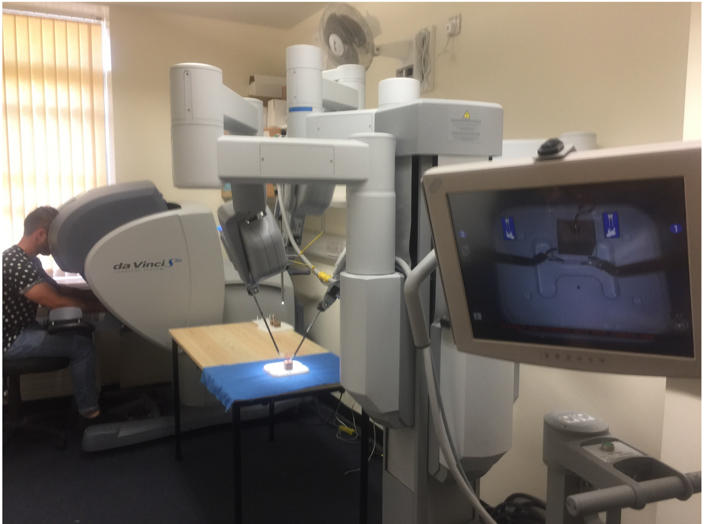
Fig 1. The DaVinci S robotic platform with surgeon console (left) and operating cart (centre).
