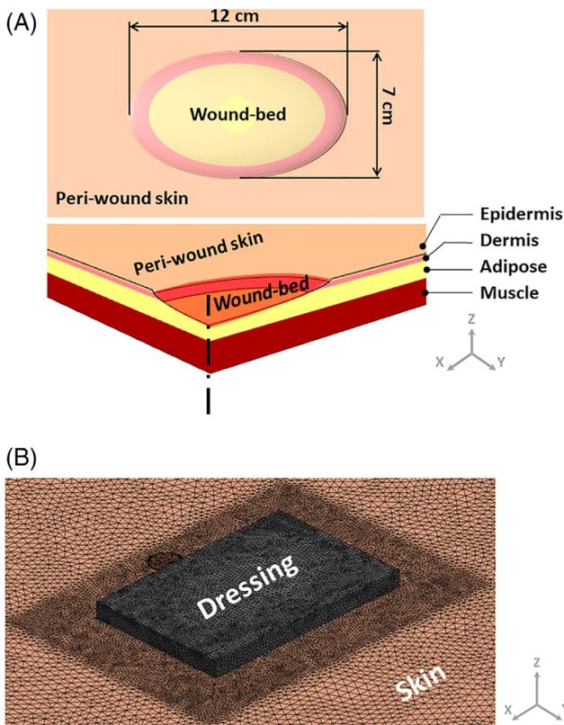
**FIGURE 3** Geometry of the computational, finite element (FE) open wound model from top and cross-sectional views A, and the FE mesh around the wound-bed with the applied dressing, showing an increased mesh density around the applied dressing for accuracy of the calculations
