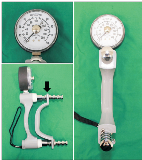
Fig. 1. Jamar Dynamometer. The Jamar and its variants use a sealed hydraulic system to measure grip strength displayed in either pounds or kilograms on an analog readout dial. The device is equipped with 2 handles and the distance between the handles can be adjusted to accommodate different hand sizes at 5 different positions. One of the handles is curved to fit the hand and the other handle position (black arrow) is used in this study, as recommended by the American Society of Hand Therapists guidelines. 3)
