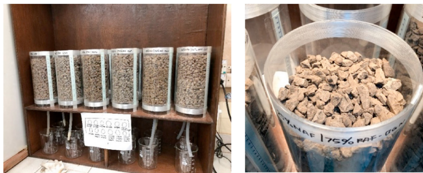
Figure 3. Column leach test (left) and the initial conditions of the sample on the surface (right).
