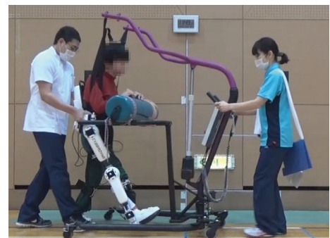
Fig. 1. Photograph of the gait training using a hybrid assistive limb.
