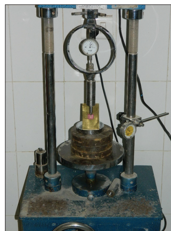
Figure 3: Specimen in inclined mold loaded with force in the universal testing machine
