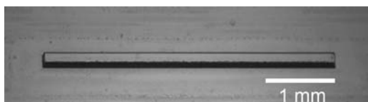
Figure 1. A mould for microchannel machined into PMMA using a micromilling machine.
