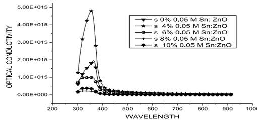
Fig. 8. The optical conductivity of 0.05 M Sn-doped ZnO.
