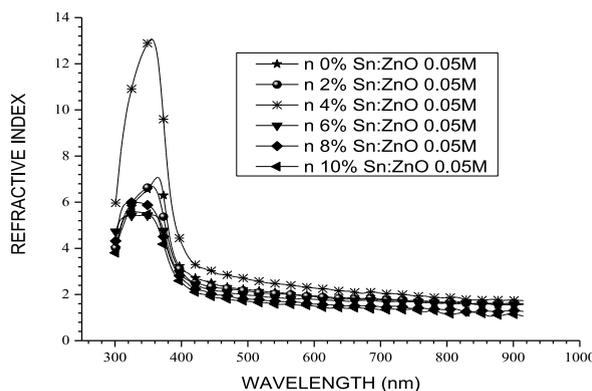
Fig. 4. The refractive index of 0.05 M Sn-doped ZnO.
