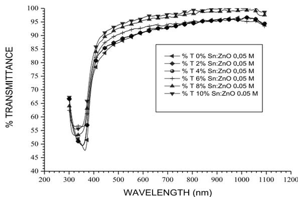
**Fig. 2.** Optical transmittance of 0.05 M Sn–ZnO thin films.
