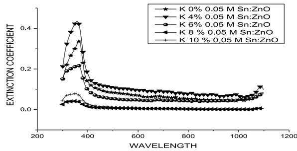
Fig. 5. The extinction coefficient of 0.05 M Sn-ZnO.
