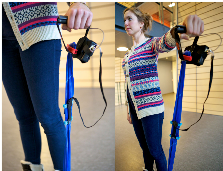
Figure 1. Elastic exercise band with the stretch sensor attached.
