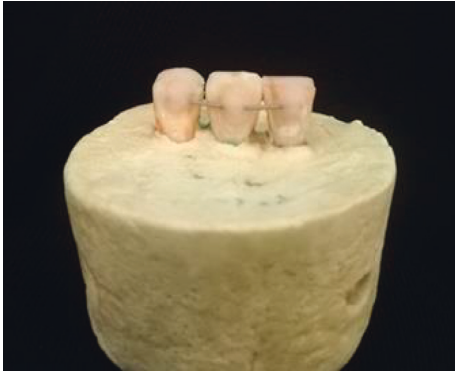
FIGURE 1: Mounting of the teeth in sets of three.
