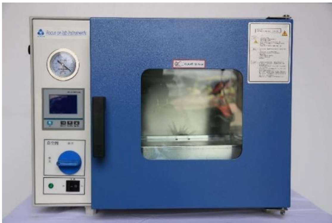
Figure 4. Vacuum chamber and high-temperature curing equipment.
