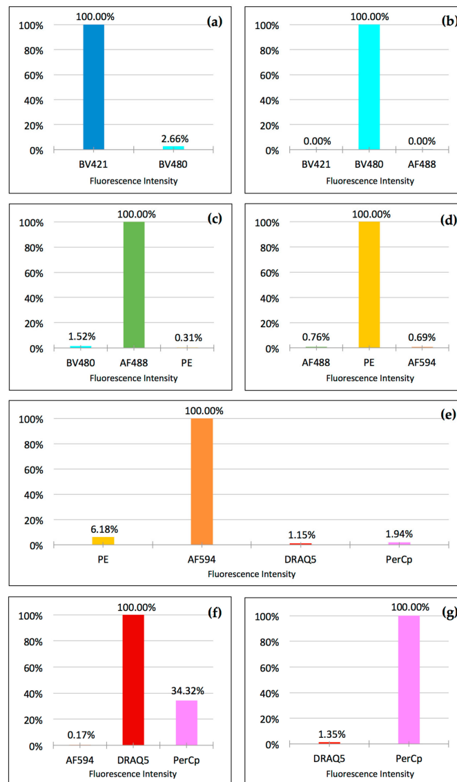
Figure 3. Crosstalk depicted for each fluorophore: Fluorescence intensity of each respective main channel is set to 100%. Crosstalk into adjacent channels is shown as percentage of fluorescence intensity of the main channel. (a) Brilliant Violet 421; (b) Brilliant Violet 480; (c) Alexa Fluor 488; (d) PE; (e) Alexa Fluor 594; (f) DRAQ5; and (g) PerCp. Cells were stained on separate slides for each fluorophore and data was acquired on a Leica DM6000B microscope with a 40× objective and 0.63× camera adapter using the 12-bit setting of a monochrome Hamamatsu Orca R2 digital camera. Integrated fluorescence density was determined after the subtraction of background fluorescence in each channel. Data are from at least six cells per channel. Standard deviation was minimal with error bars too small to show. Channels not shown did not exhibit detectable crosstalk.
