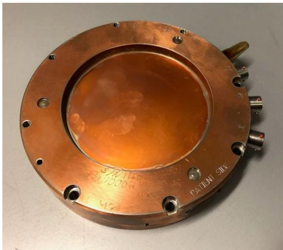
**FIGURE 1** Kapton monitor chamber (P/N100029495-02) used in Varian TrueBeam
