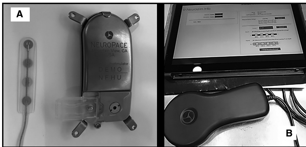
Fig. 1 (A) The neurostimulator and a strip lead. (B) The tablet for physician use and the wand used to access the neurostimulator.
