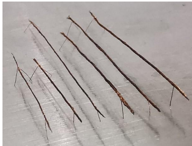
Figure 15. Different masses of manufactured beam-shaped copper wire weights.
