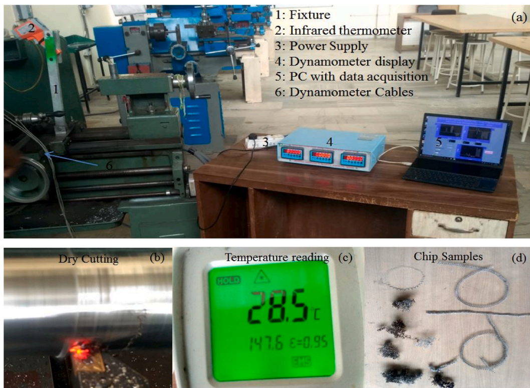
Fig. 4. (a) Measurement of cutting forces; (b) dry machining; (c) Temperature indicator; (d) Chip samples.
