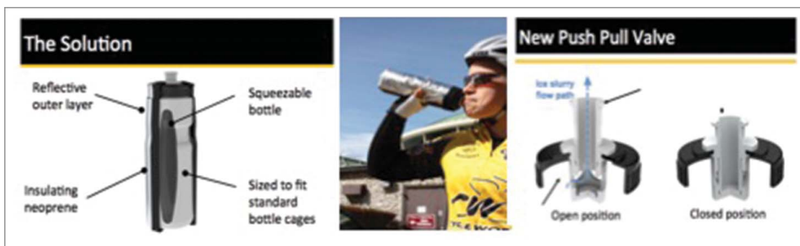
Figure 3. Prototype bottle developed by the 4 th year Engineering students at the University of Canterbury. Pictures owned by the author.
