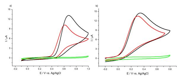
**Figure 3.** CVs of bare GCE (red) and 1% HMT-PMBI-coated electrode (black) recorded in 1 mM UA at pH 7 (a) and 1 mM AA at pH 4 (b); supporting electrolyte: 0.1 M NaCl; scan rate of 50 mV·s<sup>-1</sup>. The curve in green represents the blank CV of GCE recorded in supporting electrolyte only.
