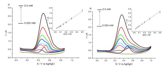
Figure 6. DPVs of bare GCE (a) and of 1% HMT-PMBI (b)-coated electrode recorded in 0.1 M NaCl supporting electrolyte in the presence of constant 0.01 mM UA and various concentrations of AA, from 25  $\mu$ M to 0.5 mM. Scan rate of 10 mV·s<sup>-1</sup>. Inset: plot of peak currents vs. concentration of AA.
