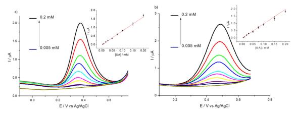
**Figure 9.** DPVs of bare GCE (a) and of 1% HMT-PMBI-coated electrode (b) recorded in Surine<sup>®</sup> in the presence of various concentrations of UA, from 5  $\mu$ M to 0.2 mM. Scan rate of 10 mV·s<sup>-1</sup>. Inset: plot of peak currents vs. concentration of UA.
