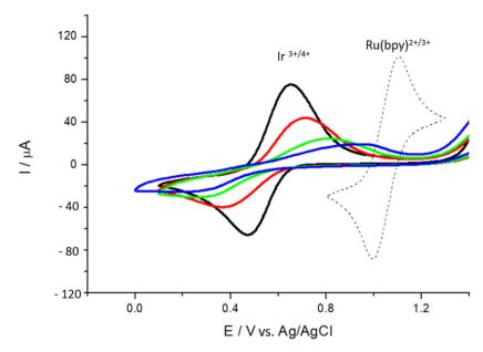
**Figure 2.** CVs of 1% HMT-PMBI-coated film loaded in 3 mM  $\rm K_4IrCl_6$  after transferring to 0.1 M NaCl supporting electrolyte, and with the addition of different concentrations of Ru(bpy)<sub>3</sub><sup>2+</sup>: 0.1 mM (black); 5 mM (red), 15 mM (green) and 30 mM (blue). Dashed CV: bare GCE recorded in 10 mM Ru(bpy)<sub>3</sub><sup>2+</sup>; scan rate of 100 mV·s<sup>-1</sup>.
