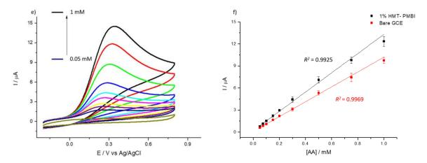
**Figure 4.** CVs of bare GCE (**a**,**d**) and of 1% HMT-PMBI (**b**,**e**)-coated electrode recorded in 0.1 M NaCl supporting electrolyte in the presence of various concentrations of UA from 5  $\mu$ M to 0.2 mM (**a**,**b**) and AA from 5  $\mu$ M to 1 mM (**d**,**e**). Scan rate of 50 mV s<sup>-1</sup>. Plot of peak currents vs. concentration of UA (**c**) and AA (**f**); bare GCE (red line), HMT-PMBI-coated electrode (black line).
