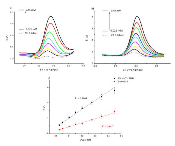
**Figure 10.** DPVs of bare GCE (a) and of 1% HMT-PMBI-coated electrode (b) recorded in Vitamin C tablet in the presence of various concentrations of AA, from 25  $\mu$ M to 450 mM. Scan rate of 10 mV·s<sup>-1</sup>. Plot of peak current vs. concentration of AA (c); bare GCE (red line), HMT-PMBI-coated electrode (black line).
