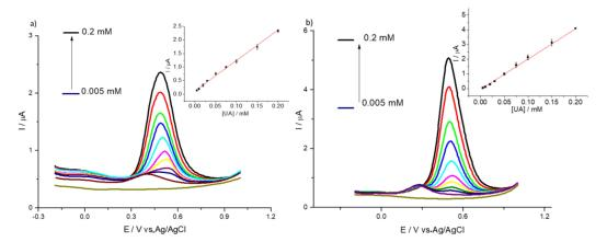
Figure 7. DPVs of bare GCE (a) and of 1% HMT-PMBI (b)-coated electrode recorded in 0.1 M NaCl supporting electrolyte in the presence of constant 0.05 mM AA and various concentrations of UA, from 5  $\mu$ M to 0.2 mM. Scan rate of 10 mV s<sup>-1</sup>. Inset: plot of peak currents vs. concentration of UA.
