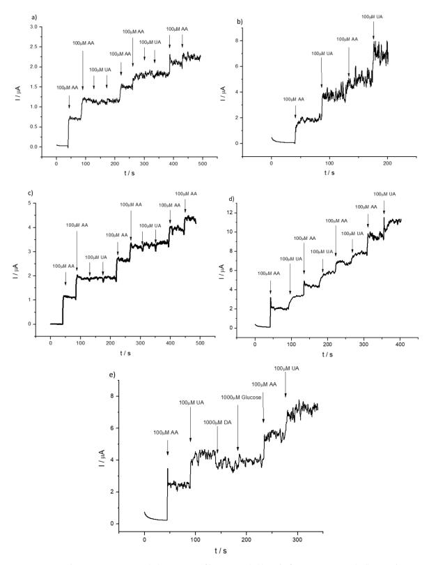
**Figure 8.** Chronoamperometric (i-t) response of bare GCE (**a**,**b**) and of 1% HMT-PMBI (**c**,**d**)-coated GCE applying 0.3 V and 0.6 V obtained with successive concentration of 100  $\mu$ M UA and 100  $\mu$ M AA from recorded in 0.1 M NaCl supporting electrolyte (pH 7) (**e**) 1% HMT-PMBI applying 1 V and adding concentrations of UA, AA, DA and glucose.
