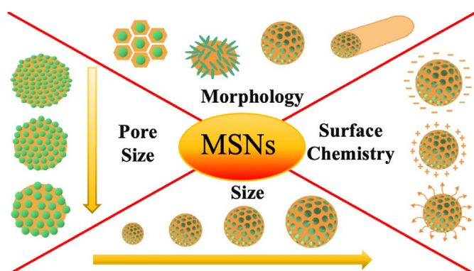
Fig. 2. Schematic illustration of tunable physicochemical properties of MSNs.
