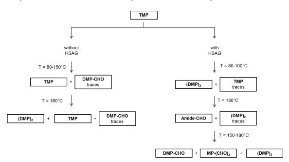
**Figure 8.** Scheme for the formation of TMP derivatives after thermal treatments at different temperatures, in the absence and in the presence of a catalytic amount of HSAG, from <sup>1</sup>H NMR analysis of the liquid fraction.
