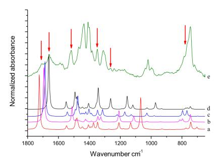
**Figure 4.** DFT computed spectra of: DMP-COOH (a), MP-(CHO)<sub>2</sub> (b), DMP-CHO (c), and DMP-COOH H-bonded dimer (d). The experimental reference spectrum (e) of modified TMP (sample treated at 130  $^{\circ}$ C in the absence of HSAG, spectrum recorded after TMP evaporation) is reported, where red arrows indicate absorption features, which can be rationalized with the occurrence of the oxidized species.
