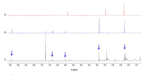
**Figure 5.** <sup>1</sup>H NMR spectra (400 MHz, CDCl<sub>3</sub>) of pristine TMP (**a**), DMP-CHO (see Table 2) (**b**), liquid product obtained by heating TMP in the presence of catalytic amount of HSAG at 150  $^{\circ}$ C (**c**). The arrows indicate the peaks assigned to DMP-CHO.
