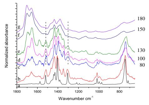
**Figure 10.** Experimental spectra of: (a) TMP, (b) reference spectrum of TMP sample treated in air at 130 °C (residue after evaporation), (c)–(g) solid powder of HSAG/TMP mixture in equimolar amount treated at different temperature.
