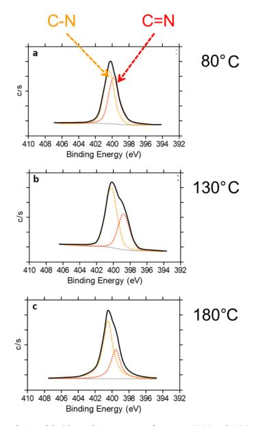
**Figure 12.** Deconvolution of the N1s peak into two contributions, at 398.9 and 400.3 eV, attributed to  $C(sp^2)N$  (N=C) and  $C(sp^3)N$  (N–C) bonds, respectively, for HSAG/TMP equimolar adducts treated at 80 °C (**a**), 130 °C (**b**), 180 °C (**c**).
