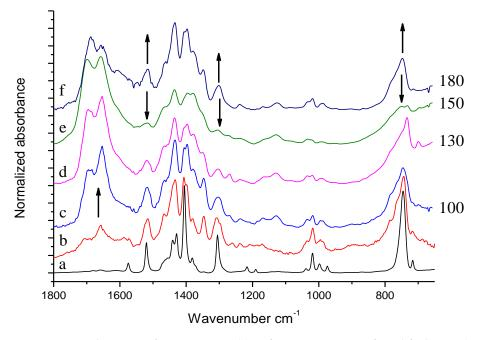
**Figure 9.** Experimental spectra of pristine TMP (**a**), reference spectrum of modified TMP (sample treated at 130 °C-residue after evaporation)) (**b**), solid powder of HSAG/TMP mixture isolated after the reaction of TMP with the catalytic amount of HSAG (**c**)–(**f**). On the right side of the Figure, treatment temperatures (°C) are indicated.
