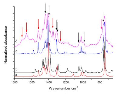
**Figure 6.** DFT computed spectrum of: TMP (**a**) and of  $\alpha$ - $\alpha'$  dimer of TMP (DMP)<sub>2</sub> (**b**). Experimental spectra of pristine TMP (**c**) and the reference spectrum of modified TMP-sample treated at 130 °C in the absence of HSAG, spectrum recorded after TMP evaporation (**d**). Black and red arrows indicate absorption features which can be rationalized with the occurrence of (DMP)<sub>2</sub> and TMP oxidized species respectively.
