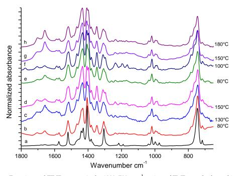
**Figure 3.** Experimental FT-IR spectra, in the 1800–700 cm<sup>-1</sup> region, of TMP samples heated in air at different temperatures. Spectra were recorded two minutes after drop deposition. On the right side of the Figure, treatment temperatures (°C) are indicated. (**a**): pristine TMP. (**b**–**d**): samples treated in the absence of HSAG. (**e**–**h**): samples treated in the presence of catalytic amount of HSAG.
