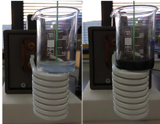
Figure 2. Experimental setup of PMF hyperthermia for HTP (left) and CTP (right) samples.
