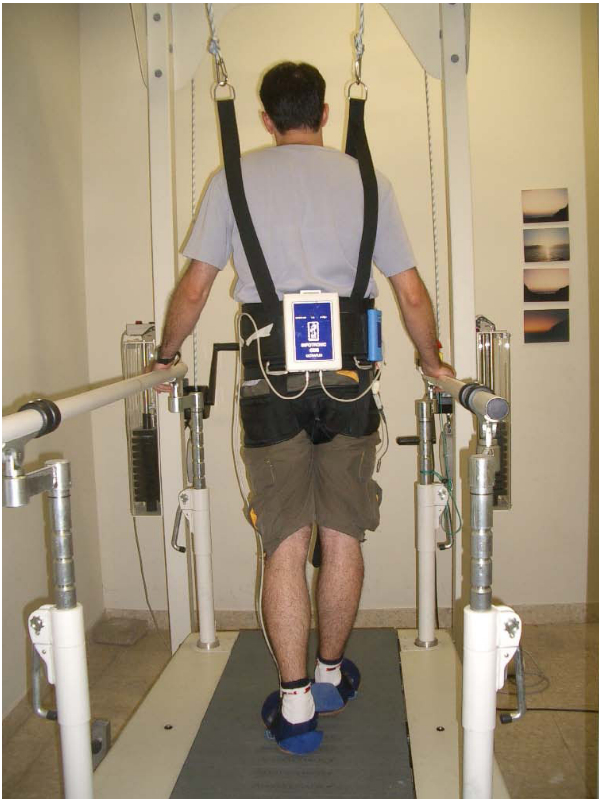
Figure 1 The setup used to assess near falls. The medical treadmill and harness used are shown along with the sensors used. A 3D accelerometer is located on the lower back and held in place by the large belt shown.
