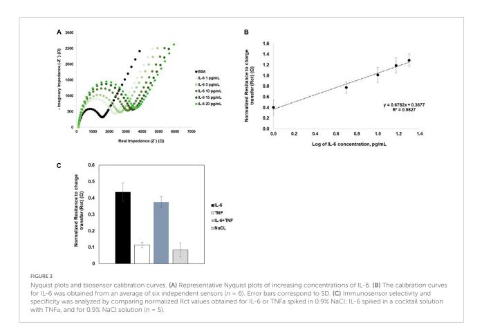
in the Nyquist plots (**Figure 3A**), with the increase in the semicircle between concentration. The IL-6 immunosensor exhibited linear range between 1 and 20 pg/mL (**Figure 3B**). The linear regression is given by y = 0.6782x+0.3677 with  $R^2 = 0.9827$ . The calculated limit of detection (LOD) was 0.088 pg/mL
