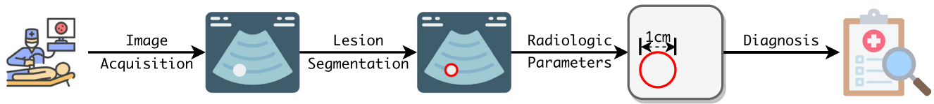
Fig. 1 | General pipeline of ultrasound image diagnosis. It usually consists of four stages: image acquisition, lesion segmentation, radiologic parameters extraction, and diagnosis.
