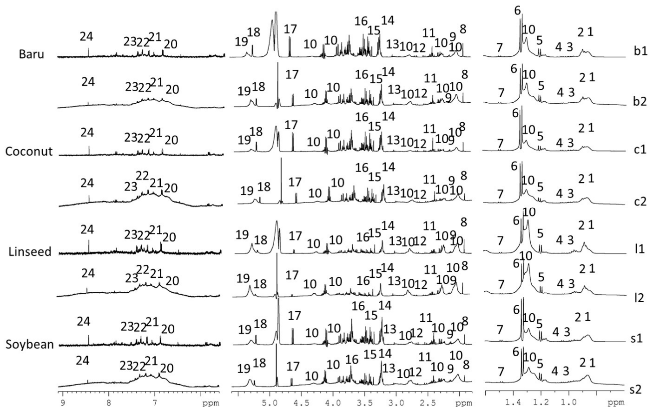
Figure 1. Representative ^1\text{H} NMR spectra (500 MHz, \text{D}_2\text{O} buffer pH 7.2) of mice serum from CPMGPR1D (b1, c1, l1, s1) and NOESYGPPR1D (b2, c2, l2, s2) pulse sequences containing the assigned metabolites: 1, 2—LDL/VLDL, 3—leucine, 4—valine, 5— \beta -hydroxybutyrate, 6—lactate, 7—alanine, 8—acetate, 9—glutamine/glutamate, 10—lipids, 11—succinate, 12—citrate, 13—creatine/creatinine, 14—choline, 15—phosphocholine, 16—taurine, 17— \beta -glucose, 18— \alpha -glucose, 19—unsaturated fatty acids, 20—tyrosine, 21—histidine, 22—L-phenylalanine, 23—tryptophan, and 24—formate.
