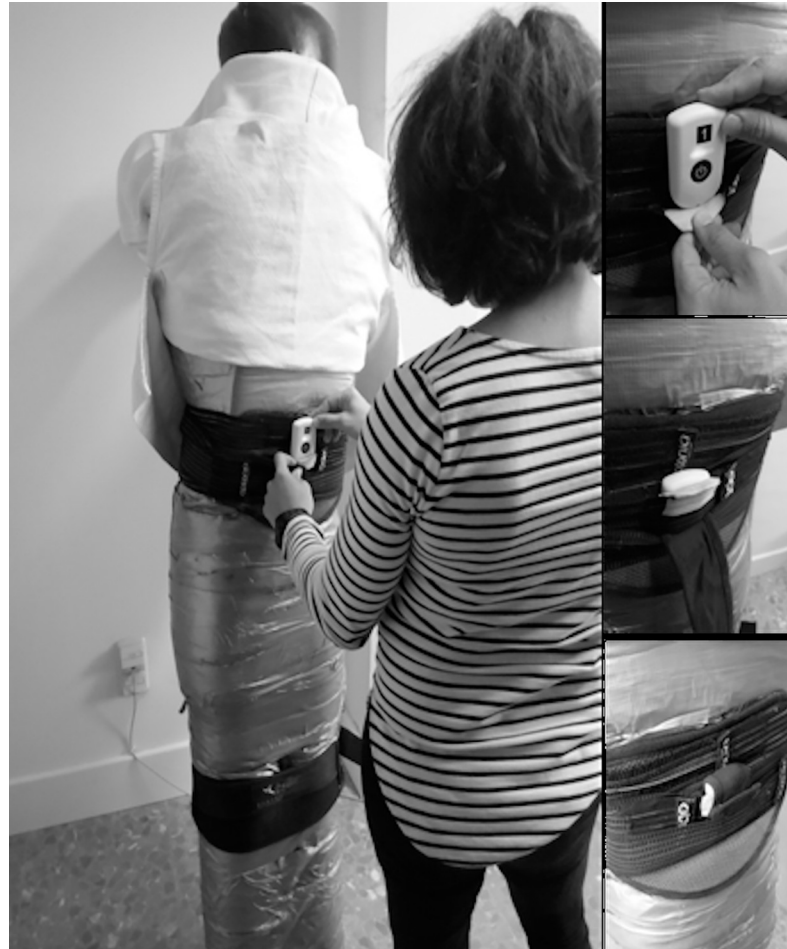
Fig 3. Placement of the wearable sensor (Wimu, Realtrack System, Almería, Spain) on the back of the dummy, fixed at waist height with a belt.
