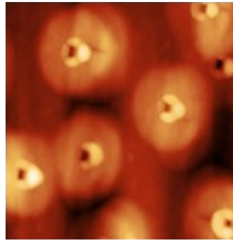
Fig. 1 AFM scan ( 1 \mu\text{m} \times 1 \mu\text{m} ) of GaAs CRDs grown on a GeTVS
