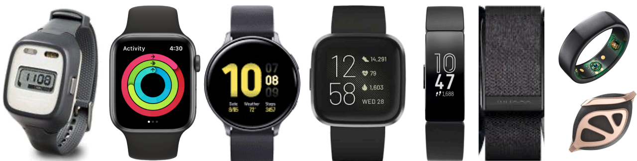
Fig. 4. Example devices used for monitoring actigraphy and physiology, including the (left to right) Actigraph Spectrum, Apple Watch, Samsung watch, FitBit Versa, Fitbit Charge, Whoop band, and jewelry based trackers, (top to bottom) Oura ring and Bellabeat Leaf. All provide basic monitoring of physical activity and heart rate, with more advanced and expensive devices offering more in-depth physiological monitoring including ECG.
