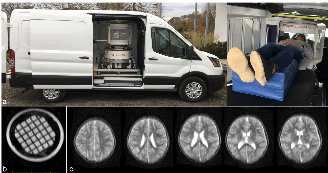
Fig. 2. Mobile low field MRI using the 64mT Hyperfine system installed in a customized cargo van (a). Despite its low field and portable nature, the device provides sound imaging abilities without geometric distortions (b) and with image quality and contrast nearing 1.5 T quality (c).
