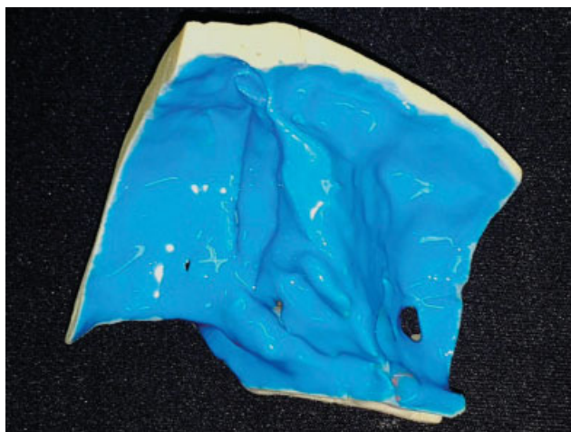
Fig. 2 Top view of the left temporal bone biomodel with blue synthetic rubber simulating the dura mater.
