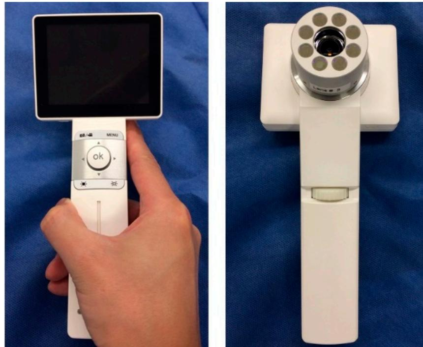
**Figure 1.** Novel handheld camera device for 5-aminolevulinic acid photodynamic diagnosis (ALA-PDD).
