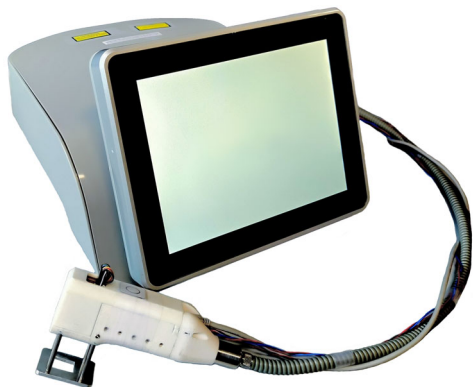
FIGURE 1 Photograph of the prototype ablative fractional fiber laser pumped DFG system. The small footprint base unit has output wavelengths of 1030 and 1560 nm, which are fiber delivered to a scanner handpiece. The scanner handpiece contains DFG crystals that convert the laser light wavelength to 3050 and 3200 nm (ratio of 2:1). DFG, difference frequency generation.
