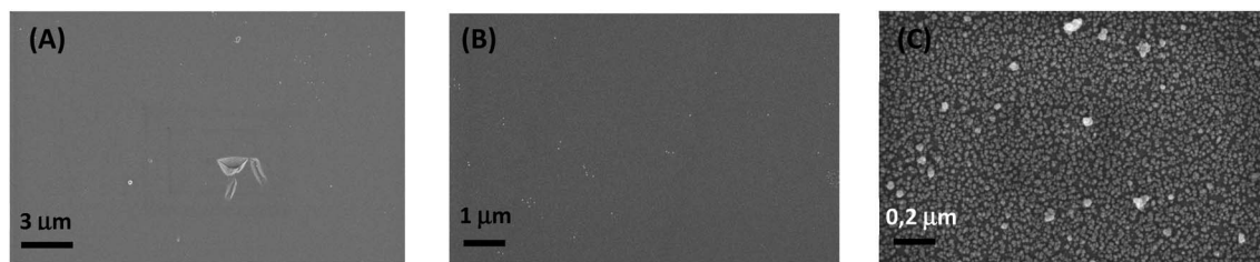
Fig. 3 Scanning electron micrographs of (A) gold surface, (B) polyethyleneimine (PEI) film and (C) PEI-supported palladium particles fabricated on Au/quartz surfaces.
